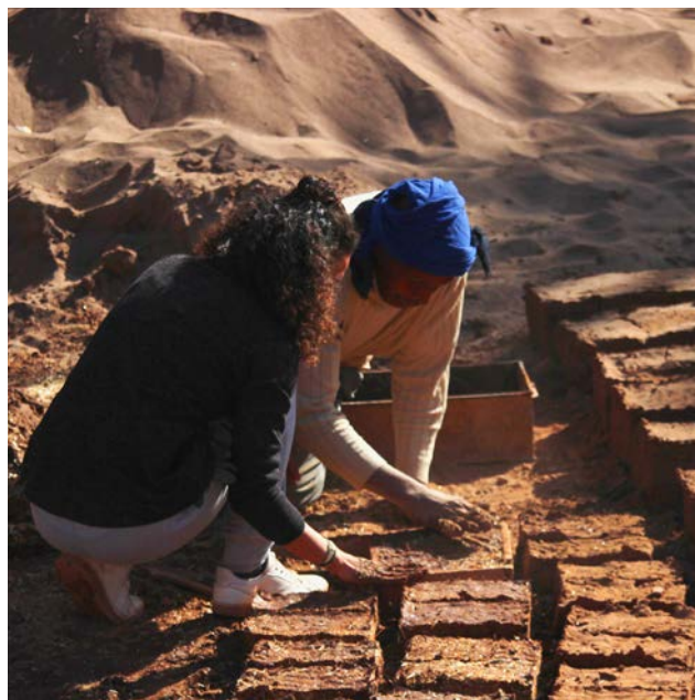
Tamping of the mud and straw mix into a wooden brick mould
