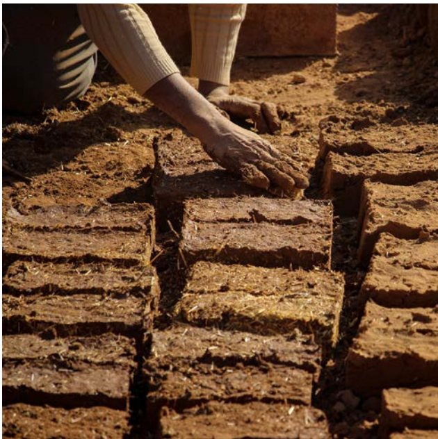
Mud bricks laid on the ground to dry in the sun
